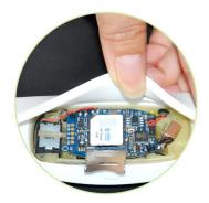
2. Open the SIM card slot, insert micro SIM card, then close the slot cover
